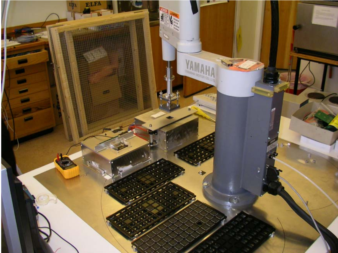
Figure 2. Photograph of the production test system for the PASA chip.
