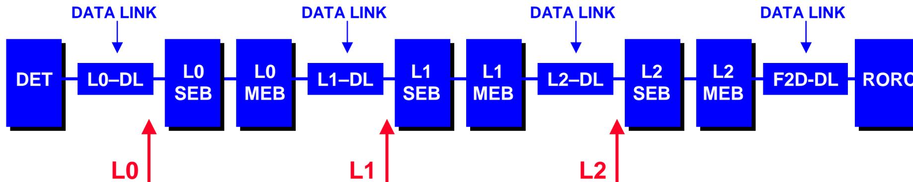
Subsequent Storage Blocks are linked by a **Data Link (DL)**. There are in general four DLs: the level-0 DL (**L0-DL**), the level-1 DL (**L1-DL**), the level-2 DL (**L2-DL**) and the Front-end to DAQ DL (**F2D-DL**). The DL is characterized by its **Transmission Latency (TL)**.
