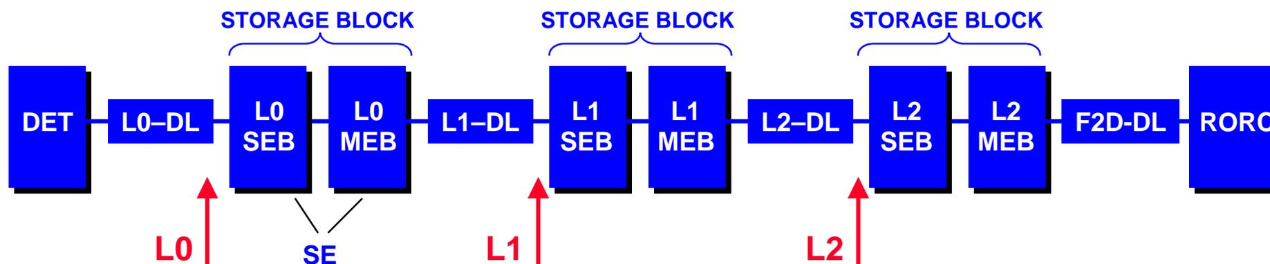
Data flows from the **Detector** (Data Source) to the **RORC** (Data Destination) through a number of analogue and digital **Storage Blocks** (SB). The Storage Blocks are organized in three levels: L0, L1 and L2. Upon arrival of the trigger signal, data is registered in the corresponding Storage Block.
