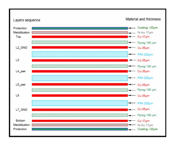
Cross section of the RCU printed circuit board. The PCB has a thickness of  $1678\mu m$  and it is the manufactured in class 6. The 8 layers of copper are interleaved with different Halogen -free dielectric materials. Note that some of the signal traces have to be implemented respecting characteristic impedance rules.
